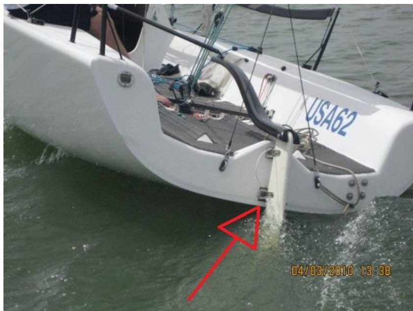
Arrow pointing to where you're gonna measure the rake
